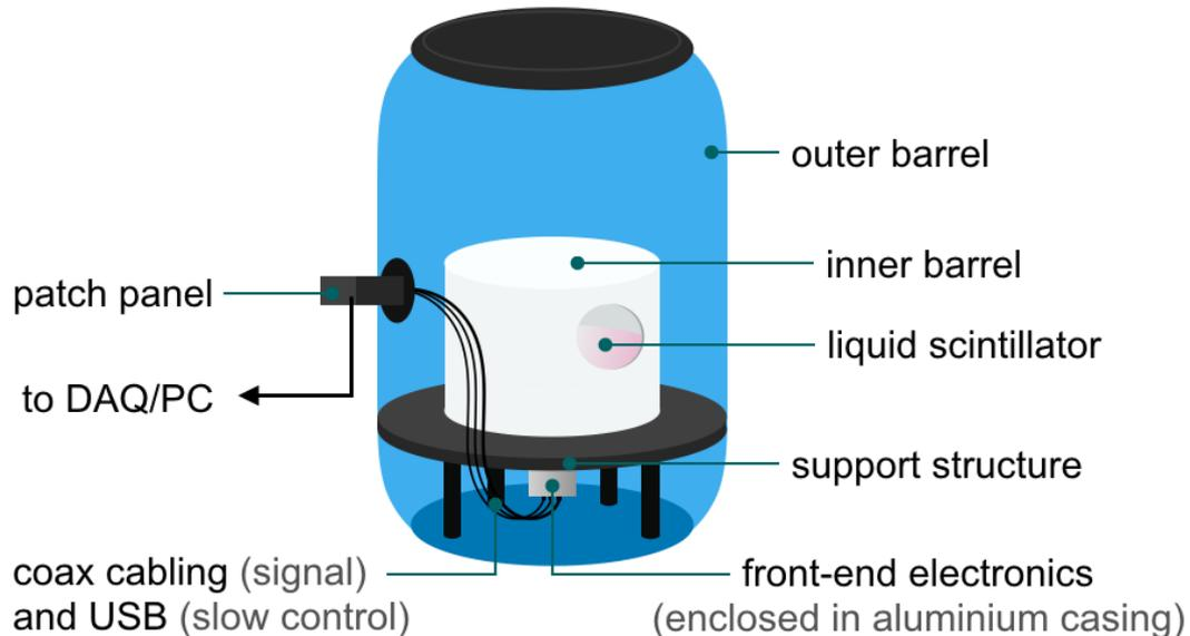
Figure 1: Basic construction of the detector used in LPT 22.
